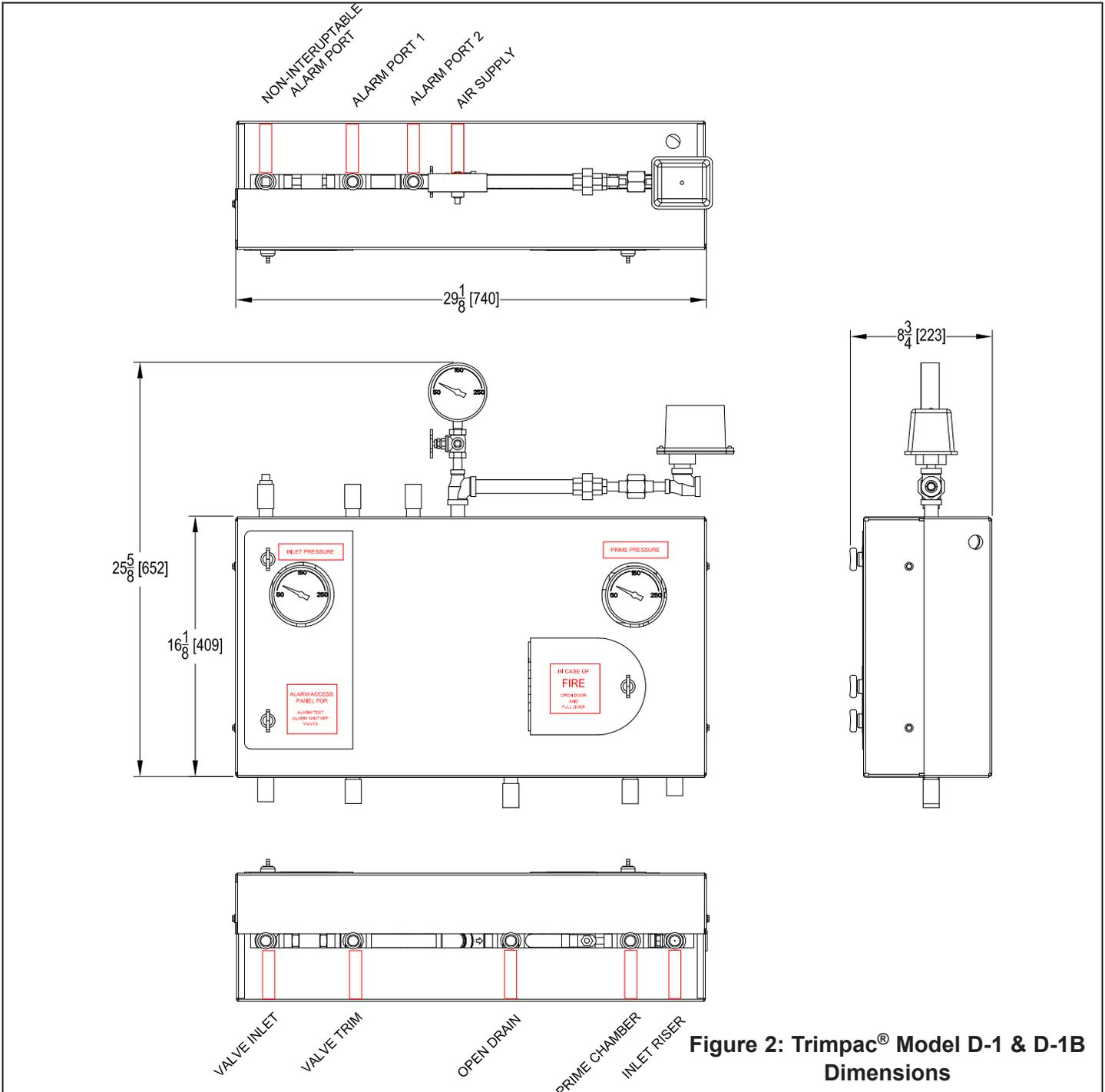
**Figure 2: Trimpac® Model D-1 & D-1B
