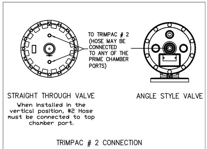
Figure 11: Valve Connections
